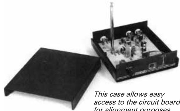
*This case allows easy access to the circuit board for alignment purposes.*
